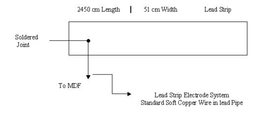
All exposed portion of the tinned copper wire and adjacent lead surfaces should be liberally coated with black paint suitable for iron work.
