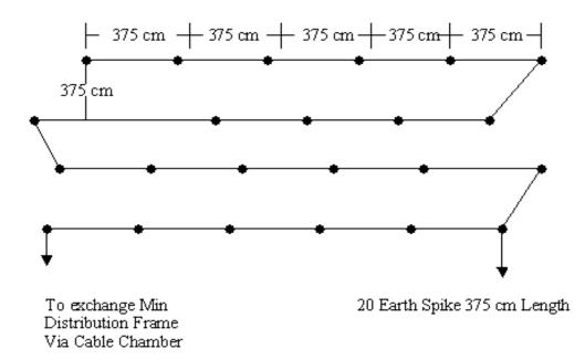
Depending upon the soil resistivity of particular place. The number and length of spike can be worked out to achieve the desired value of earth resistance.
