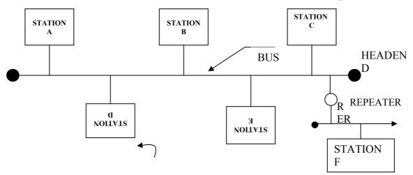
If signals are amplified along the bus, the bus becomes unidirectional. Therefore two separate channels are required. Every station injects signal on one bus and listens to the other bus. At one end of the LAN, the buses are looped. These two channels can be provided on a signal bus also using frequency division multiplexing. In this case, the head-end contains a frequency translator. Stations transmit on one frequency and listen to other frequency.
